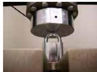
Figure 6: Force-testing of a padlock as part of ASIO's security equipment evaluation (see pg. 40).
