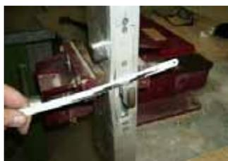
**Figure 7:** Attack testing of a mortice lock as part of ASIO's security equipment evaluation.
